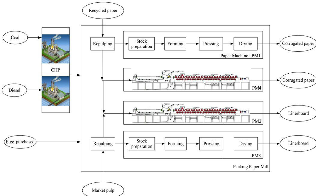
Fig. 1. Operational boundary of the packing paper mill.
