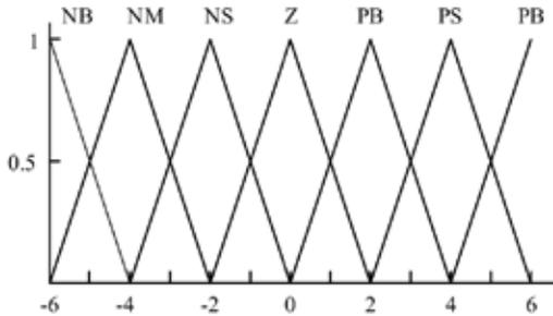
Fig. 15. Membership function curve of various  $e$ ,  $\Delta kp$ ,  $\Delta ki$ ,  $\Delta kd$ .
