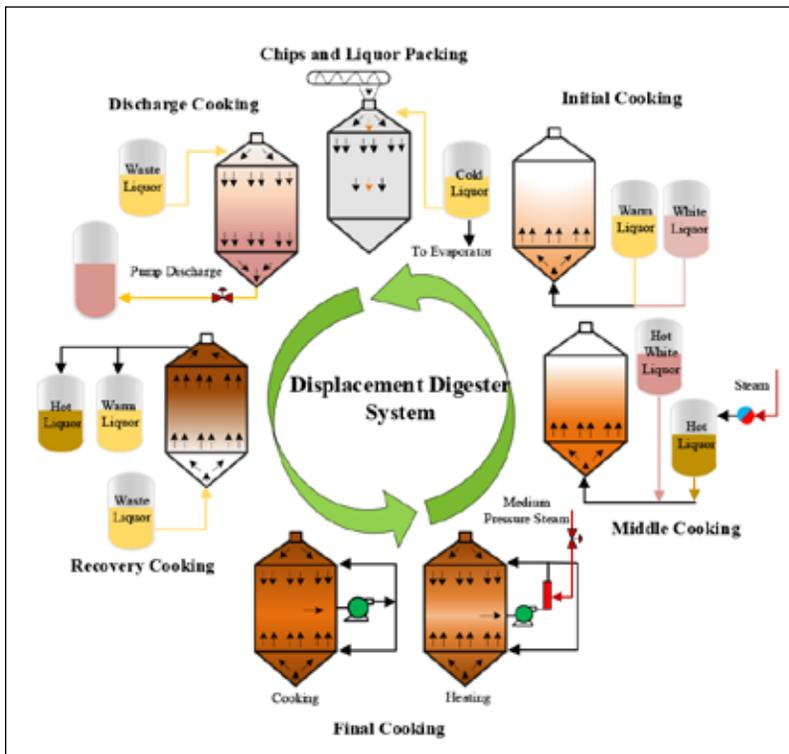
Fig. 1. Process flow chart of DDS.
