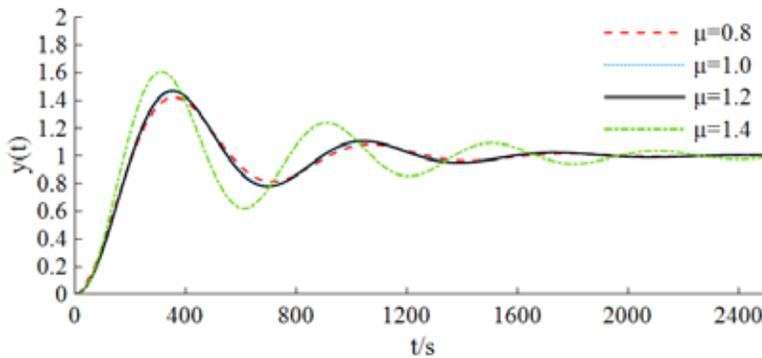
Fig. 13. Step responses of  $\mu$  with different values.
