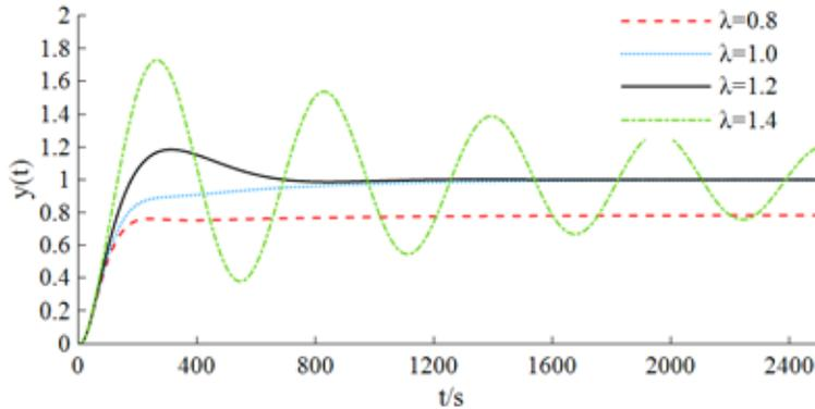
Fig. 12. Step response of  $\lambda$  with different values.
