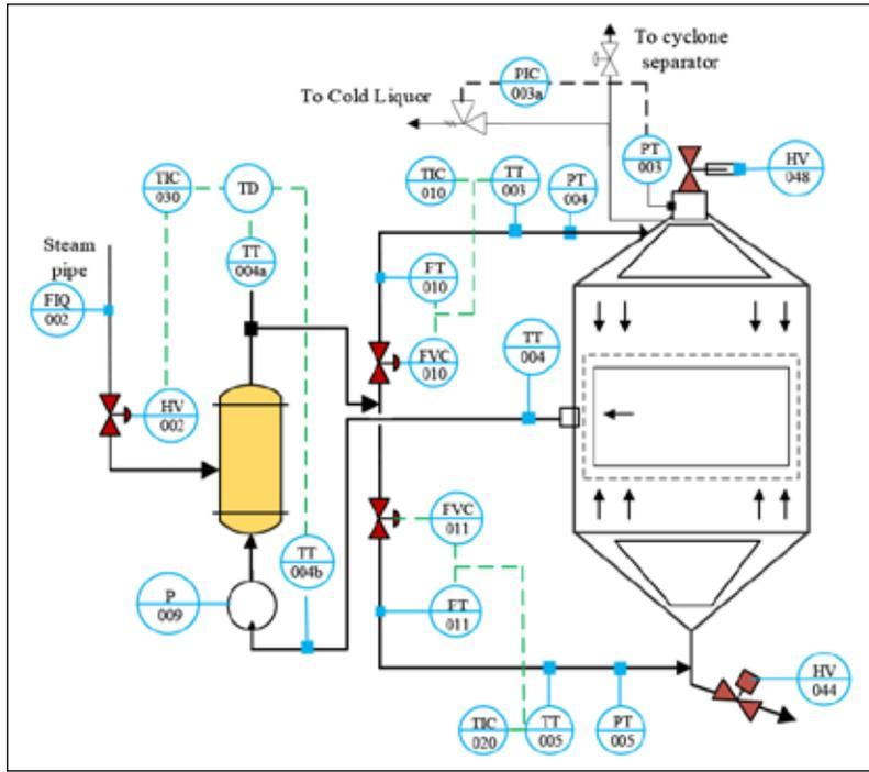
Fig. 6. Cascade Control Method of Liquor Heating.
