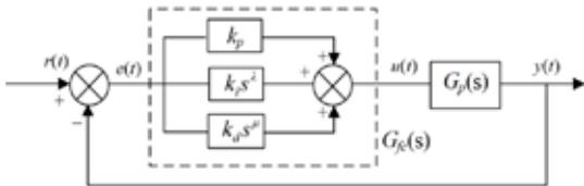
Fig. 8. Construction diagram of Fractional order PID control system.
