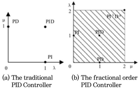
Fig. 9. Comparison of the value range of the traditional PID and fractional order PID.
