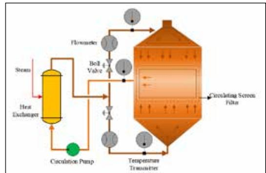
Fig. 2. The process flow of final cooking.
