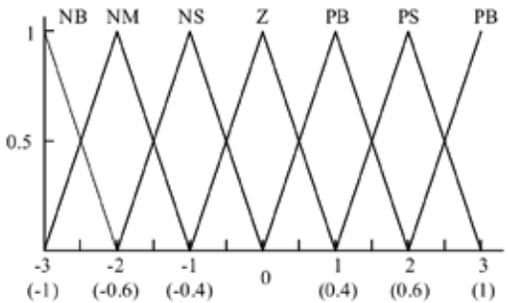
Fig. 16. Membership function curve of input variable  $ec$  (output variable  $\Delta ki$ ).
