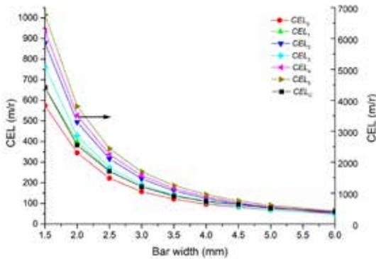
Fig. 6. The relationship between the  $CEL$  calculated by different methods and the bar width of isometric straight bar plate.
