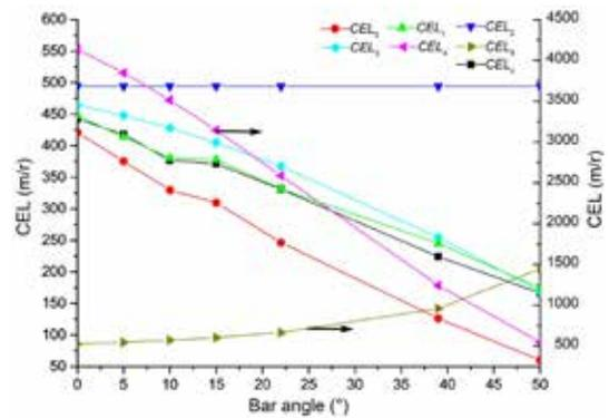
Fig. 2. The relationship between the  $CEL$  calculated by different methods and the bar angle of isometric straight bar plate.
