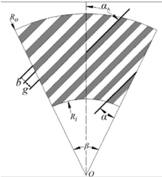
Fig. 1. Main parameters of the straight bar plates.
