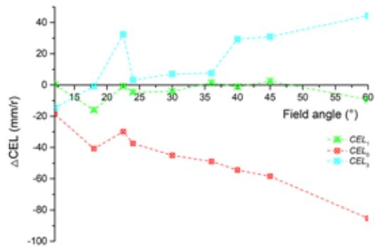
Fig. 5. The deviation of  $CEL_0$ ,  $CEL_1$ ,  $CEL_3$  and  $CEL_C$  over field angle of the straight bar plates.
