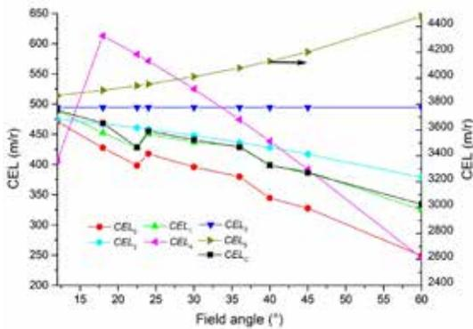
Fig. 4. The relationship between the  $CEL$  calculated by different methods and the field angle of isometric straight bar plate.
