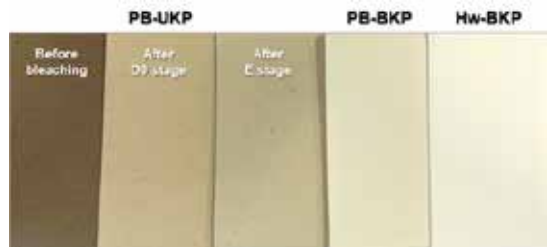
Fig. 3. Color comparison of handsheets made from PB-UKP, PB-BKP by bleaching steps and commercial Hw-BKP.
