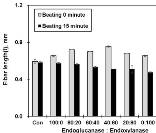
Fig. 1. Fiber length of pulp fibers depending on enzyme composition and beating.
