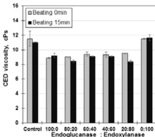
Fig. 5. CED viscosity of pulp fibers depending on enzyme composition and beating.
