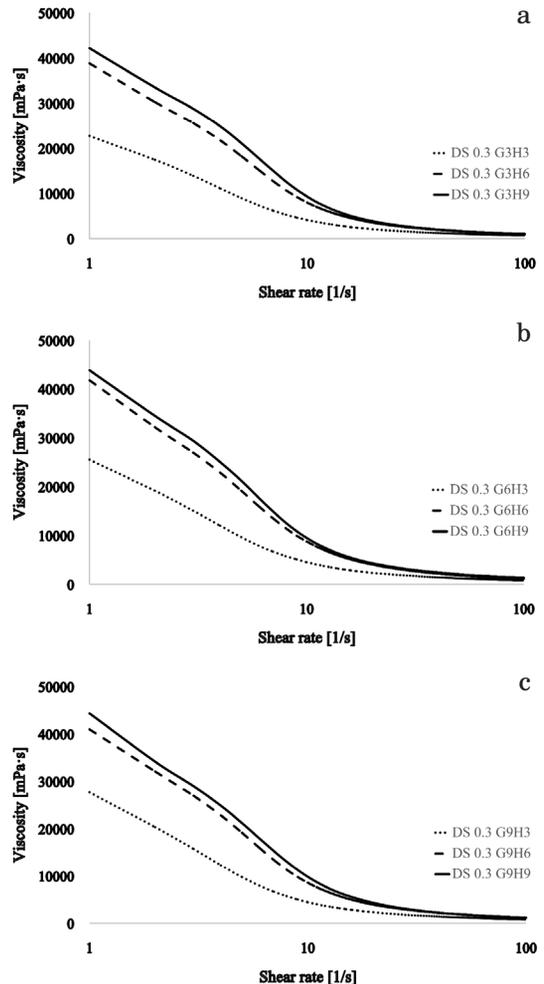
Fig. 2. Viscosity as a function of shear rate for bleached rice hull DS 0,3 CNF with different nanofibrillation combinations, three grinding passes, and different HPH passes. a) 3 HPH passes, b) 6 HPH passes, c) 9 HPH passes.
