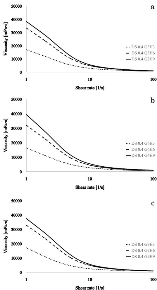
Fig. 3. Viscosity as a function of shear rate for bleached rice hull DS 0.4 CNF with different nanofibrillation combinations, three grinding passes, and different HPH passes, a) 3 HPH passes, b) 6 HPH passes, c) 9 HPH passes.
