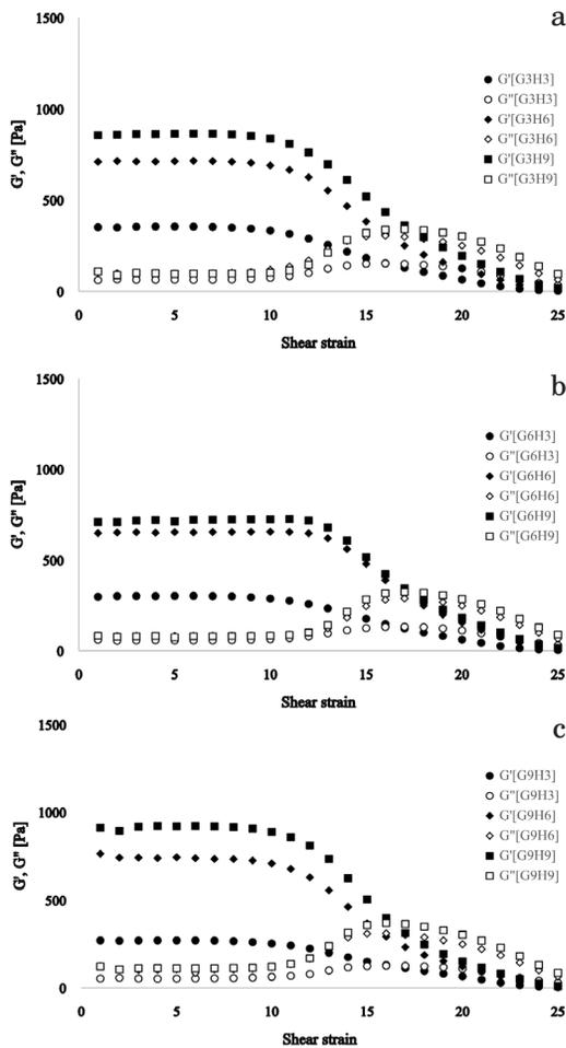
Fig. 6. Storage and loss modulus as a function of strain amplitude at a frequency of 10 rad/s for bleached rice hull DS 0.4 with 3 grinding passes and different nanofibrillation combinations a) 3 HPH passes, b) 6 HPH passes, c) 9 HPH passe.
