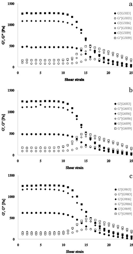
Fig. 4. Storage and loss modulus as a function of strain amplitude at a frequency of 10 rad/s for bleached rice hull DS 0.2 with 3 grinding passes and different nano-fibrillation combinations a) 3 HPH passes, b) 6 HPH passes, c) 9 HPH passes.
