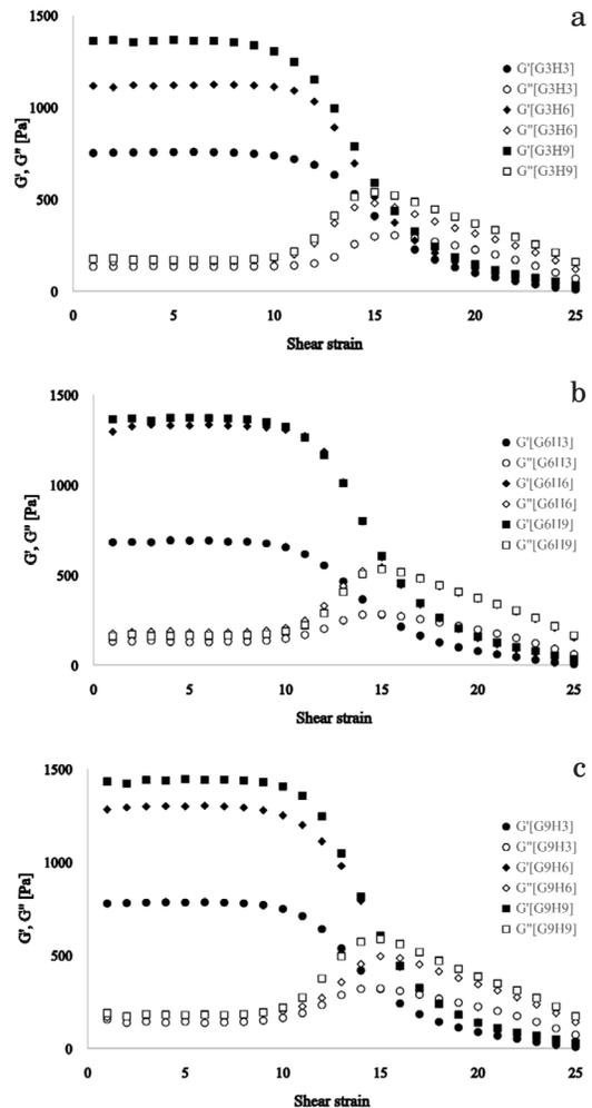
Fig. 5. Storage and loss modulus as a function of strain amplitude at a frequency of 10 rad/s for bleached rice hull DS 0.3 with 3 grinding passes and different nano-fibrillation combinations a) 3 HPH passes, b) 6 HPH passes, c) 9 HPH passes.
