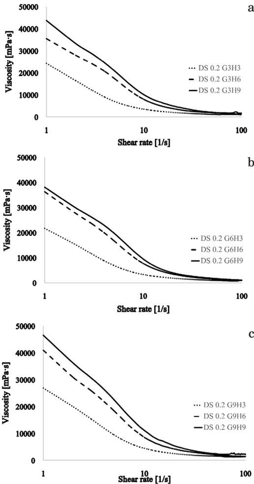
Fig. 1. Viscosity as a function of shear rate for bleached rice hull DS 0,2 CNF with different nanofibrillation combinations, three grinding passes, and different HPH passes. a) 3 HPH passes, b) 6 HPH passes, c) 9 HPH passes.
